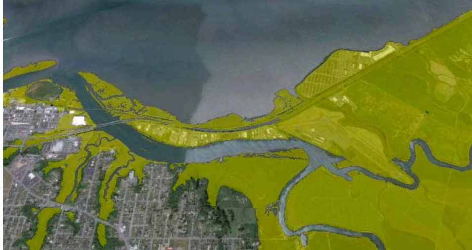
Figure Climate-4. US 101 Eureka to State Route 255 Possible Inundation
