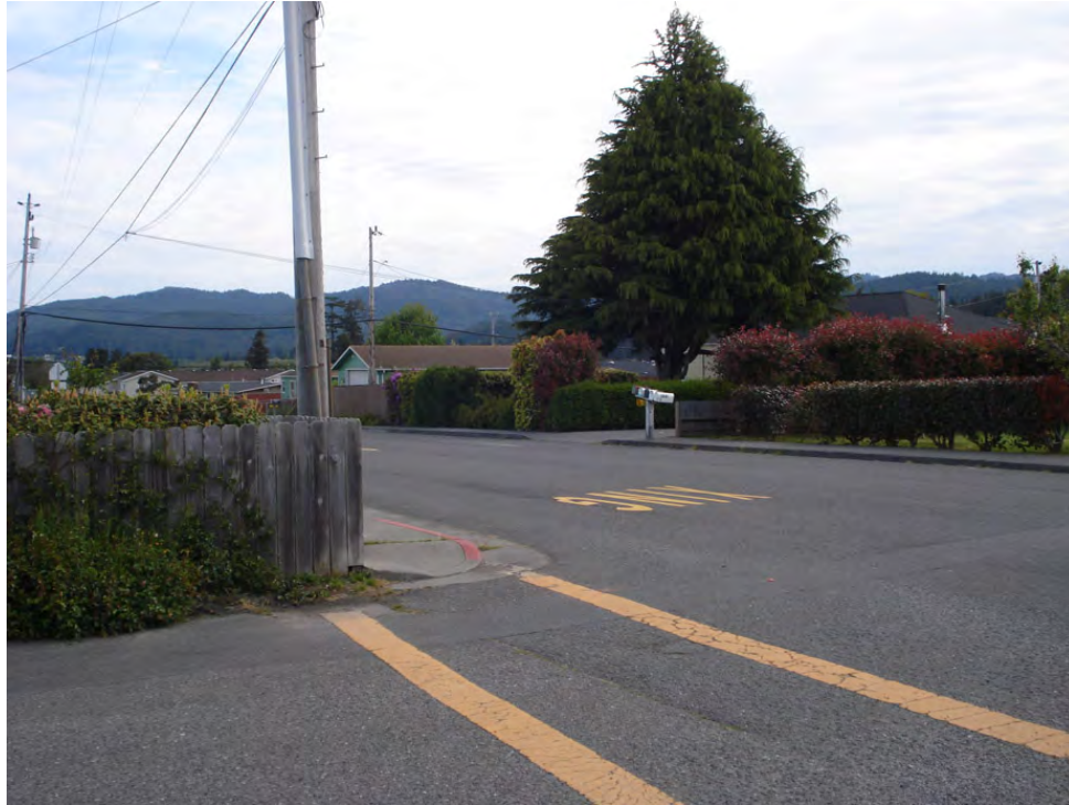
This fence location results in poor visibility next to the crosswalk on Wood and Thomas Streets.
