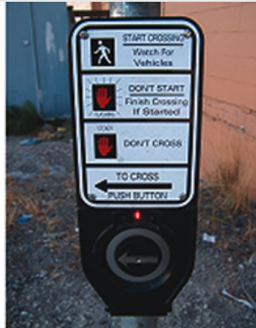
User-activated signals (ped heads). User-activated bicycle/pedestrian signals at intersections (typically only major)
