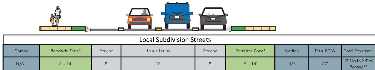
Figure 5.3-6 Typical Local Subdivision Street Cross-section
